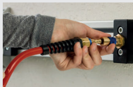
To disconnect, pull back the coupling sleeve.
