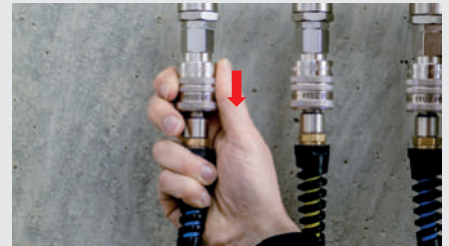
Disconnection - second step: Safe decoupling
